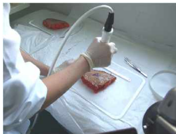
FIG. 2. Ex vivo radiofrequency application with the device's probe.
